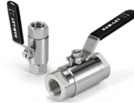
Heavy Duty Ball Valves– H-1700 Series MAWP: 6000 psi (413 bar) MAWT: 500°F (260°C)
