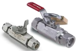
Ball Valves with Locking Device H-700 Series MAWP: 2000 psi (137 bar) MAWT: 400°F (204°C)
