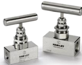
High Pressure Needle Valves H-99 Series MAWP: 10000 psi (690 bar) MAWT: 1200°F (648°C)
